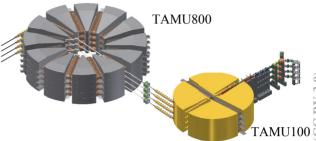
Figure 1: Accelerator system showing the four beam lines from injection through the booster and main cyclotrons.
