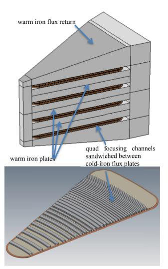
Figure 3: a) TAMU 800 sector containing apertures for 4 flux-coupled SFCs; b) detail view of one flux plate, showing the quad focusing channels and MgB<sub>2</sub> main winding.
