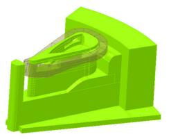
Figure 2: 3D view of the magnetic sector and of one of the pair of NbTi superconducting coils.
