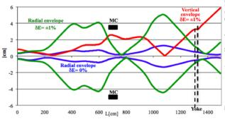
Figure 4: Radial and axial beam envelope along the extraction trajectory. Effects due to the energy spread  $(\pm 1\%)$  are also shown.
