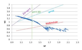
Figure 3: Tune plot of the 8-sector cyclotron.
