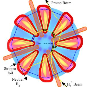
Figure 1: DSRC Layout, with the injection and extraction trajectory. Coils and cavities are also shown.
