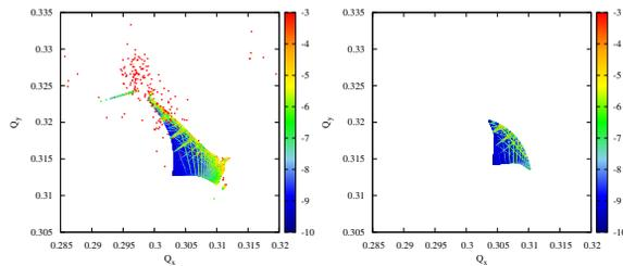
Figure 2: FMA of HL-LHC with crossing angles of  $475 \mu\text{rad}$  (left) and  $580 \mu\text{rad}$  (right) the colors illustrate the amplitude of the tune changes going from blue to red in increasing amplitude. Red indicates a tune change of  $10^{-3}$  between two samples of 2048 turns.
