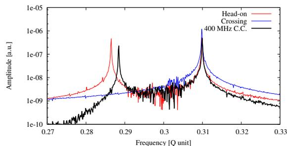
Figure 6: 6D Strong-strong simulation with and without crossing angle and crab cavities for  $\Phi \approx 3.0$ .
