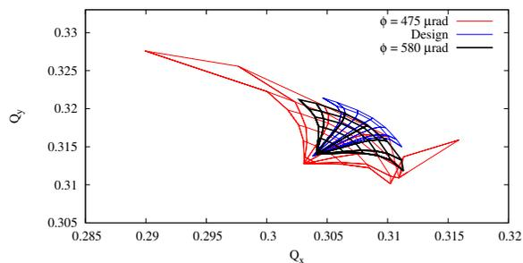
Figure 1: Tune footprints for nominal and HL-LHC beam parameters derived with MADX [8].
