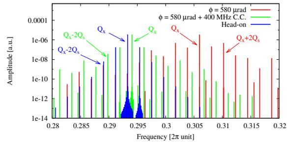
Figure 3: Horizontal spectrum comparison for head-on, crossing angle and crab compensation for a particle with initial amplitude  $1 \sigma_x$  and  $1 \sigma_s$ .
