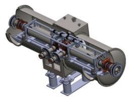
Figure 2: Schematic view of ERL main linac cryomodule.
