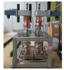
Figure 5: Fabricated input couplers for cERL main linac.
