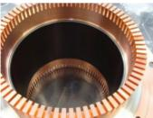
Figure 7: Ferrite and comb-structure of HOM absorber for cERL main linac.
