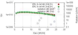
Figure 3: Vertical test results of ERL main linac 9-cell cavities. Left and right axes show  $Q_0$  and radiation dose, respectively.
