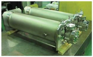
Figure 4: Main linac 9-cell cavities. After the vertical tests, He jackets were welded on them.
