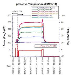
Figure 6: High power test results for cERL main linac input couplers.
