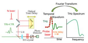
Figure 9: Schematic diagram of THz-CTR-TDS system with EO sampling method.
