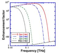
Figure 2: Enhancement factor of CSR as a function of its frequency by changing the bunch length.
