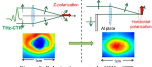
Figure 8: Polarization control of THz-CTR.
