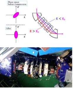
Figure 4: Magnetic bunch compressor.
