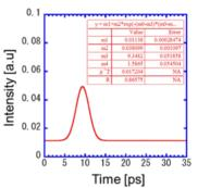
Figure 11: Measured THz temporal waveform (Gaussian fitted).
