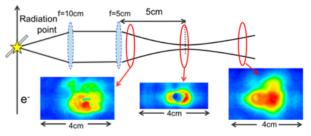
Figure 7: Profile changes of the THz-CTR electric field.
