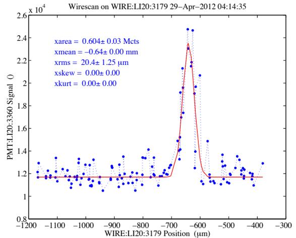
Figure 5: FACET IP Horizontal wire size 20µm.
