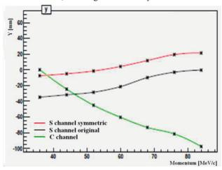
Figure 1: The mean position of the beam at the end of the bent solenoid channel in various configurations.
