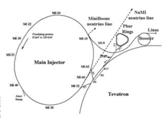
Figure 2: Layout of Fermilab Accelerator Complex.
