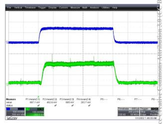
Figure 4a: Forward power (C3) and beam current (C4) signals.
