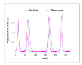
Figure 2: Field distribution in the cavity
