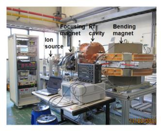
Figure 3: Experiment setup.
