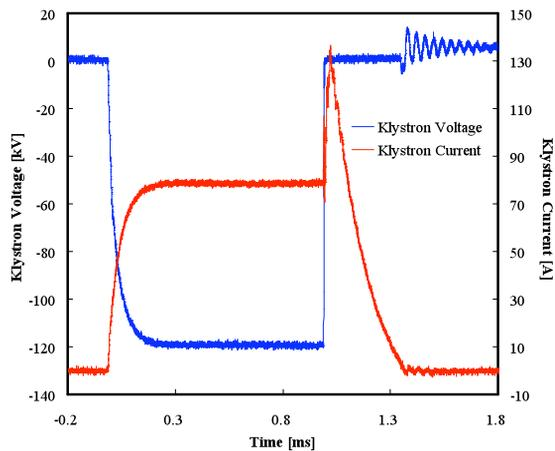
Figure 4: Klystron voltage and current waveforms during a gun spark.
