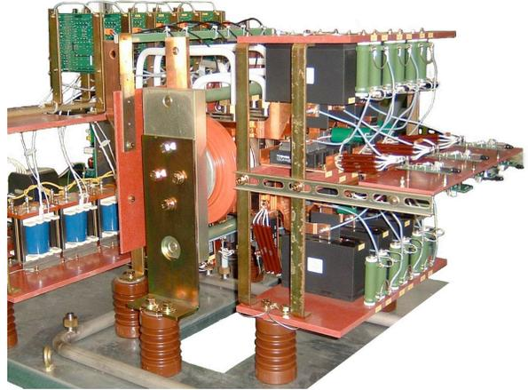
Figure 5: IEGT switch assembly.
