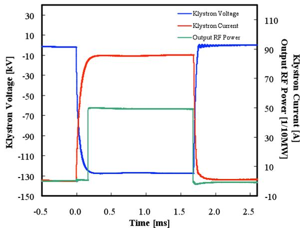
Figure 3: Klystron voltage, current and output rf power waveforms.
