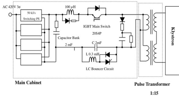
Figure 1: Simplified circuit diagram of STF modulator #2.
