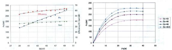
Figure 2: Characteristics of 300-kW klystron. Left: Applied voltage vs. output power (black), gain (green) and efficiency (red). Right: Input power vs. output power in various applied voltage.
