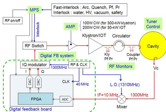
Figure 6: Block diagram of LLRF.
