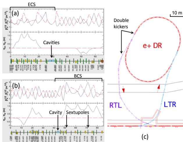
Figure 3: The  $\beta$ -functions and dispersion functions, for (a) LTR and (b) RTL. Solid (black) and dot (red) lines indicate the horizontal and vertical functions, respectively. (c) The layout of LTR, DR and RTL.
