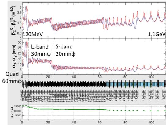
Figure 2: The  $\beta$ -functions, beam sizes (hard edge) and number of positrons after the capture section to the end of Sector 2.
