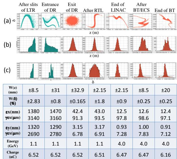
Figure 5: Distributions at the key points. (a) profiles in the longitudinal phase space, (b) histograms of  $z$ , (c) histograms of  $\delta$ . Table shows width (hard edge or  $3\sigma$ ) of  $z$  and  $\delta$ ,  $\varepsilon_x$  and  $\varepsilon_y$  with their normalized emittances, beam energy and charge intensity.
