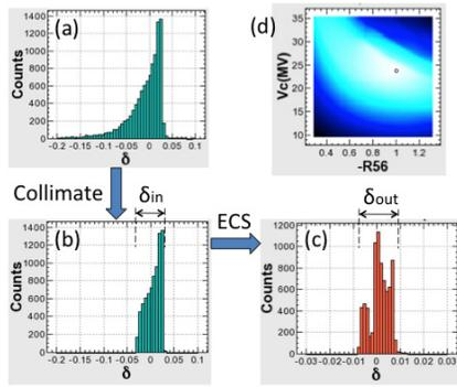
Figure 4: Distributions of beam energy spread  $\delta$  (a) at the end of Sector 2, (b) after cut by collimators at the first arc of LTR and (c) after the ECS. (d) density plots of  $R_{56}$  and  $V_c$ . Parameters at the brightest color show the largest number of particles in the momentum acceptance of the DR.
