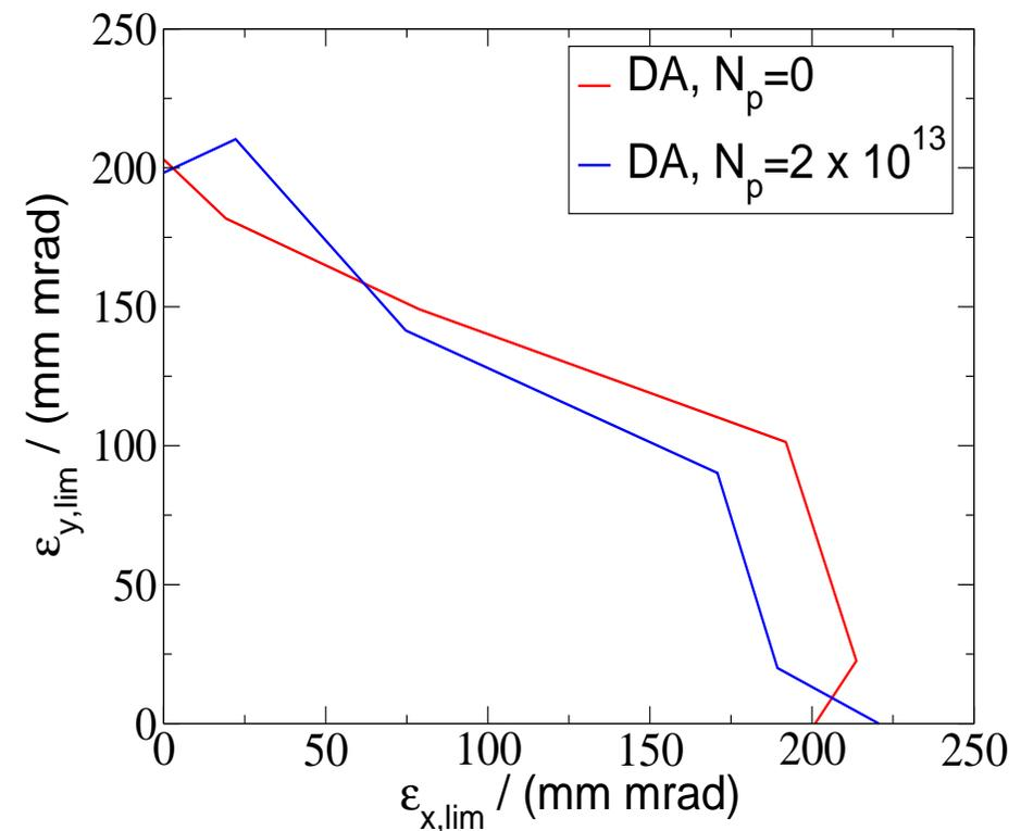
**Result:** no particle loss at  $E = 7 \text{ GeV}$ , instead ...
