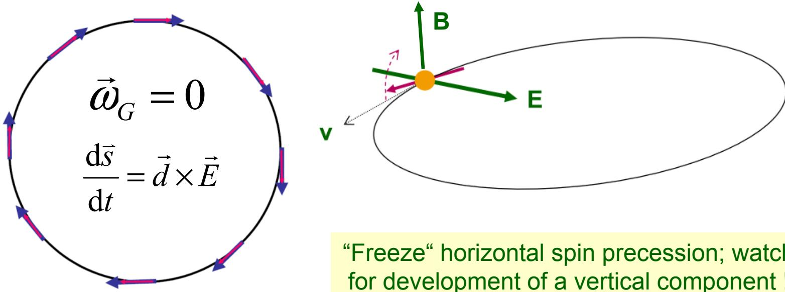
A *magic* storage ring for protons (electrostatic), deuterons, ...
