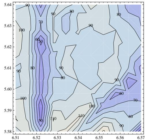
Figure 3: Luminosity versus tune of the electron ring.
