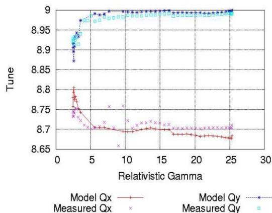
Figure 2: AGS online model tune predictions and measurements for operational currents, calculated using linear snake transfer matrices.
