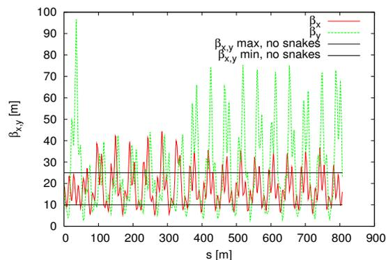
Figure 1: Modeled AGS  $\beta$  functions at injection energy with both snakes included and using operational currents in the compensation quadrupoles. Black lines show the maximum and minimum beta functions in a lattice without snakes. The compensation quadrupole currents that are ultimately determined to be optimal are often far from the modeled fit.
