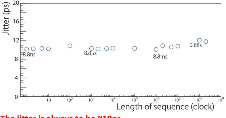
The jitter is always to be ~10ps. There is no significant difference in the length of sequence.
