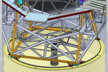
Overall view of azimuth structure with new azimuth encoder in place
