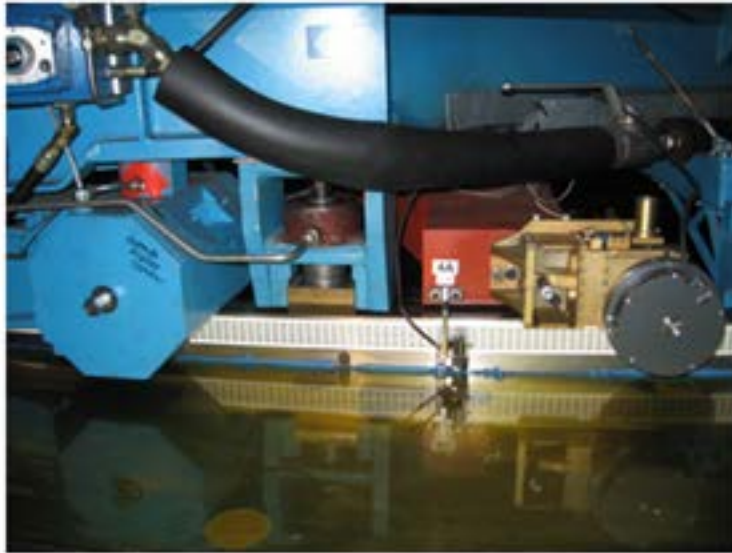
K2 Azimuth – Encoder, barcode and Precision Reference Mark (PRM)
