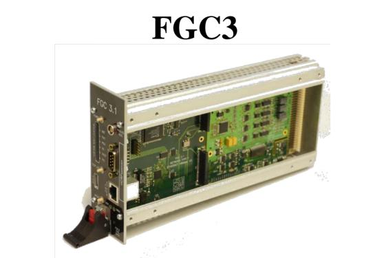
• CERN-designed power converter Function Generator / Controller.
