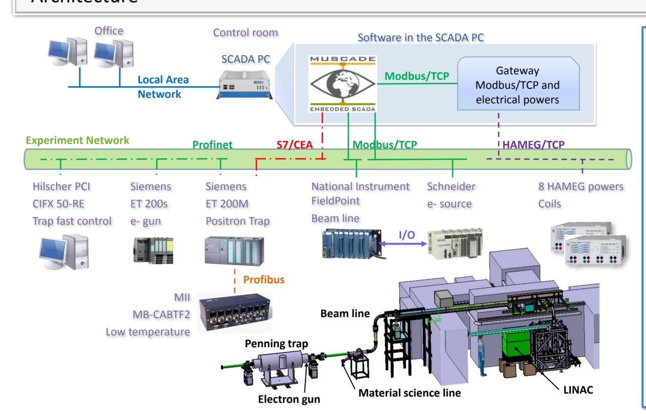
Muscade® SCADA centralizes data from the different devices and provides a graphical user interfaces (GUI) locally or from a distance (read only.)
