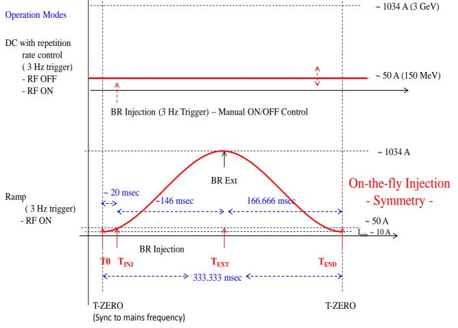
Booster synchrotron power supply waveform plans.
