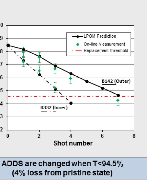
On-line (ADDS Attenuation Tool Software) transmission measurements for 192 beamlines as compared to the Laser Performance and Operations Model (LPOM) values after 1.3 MJ experiment
