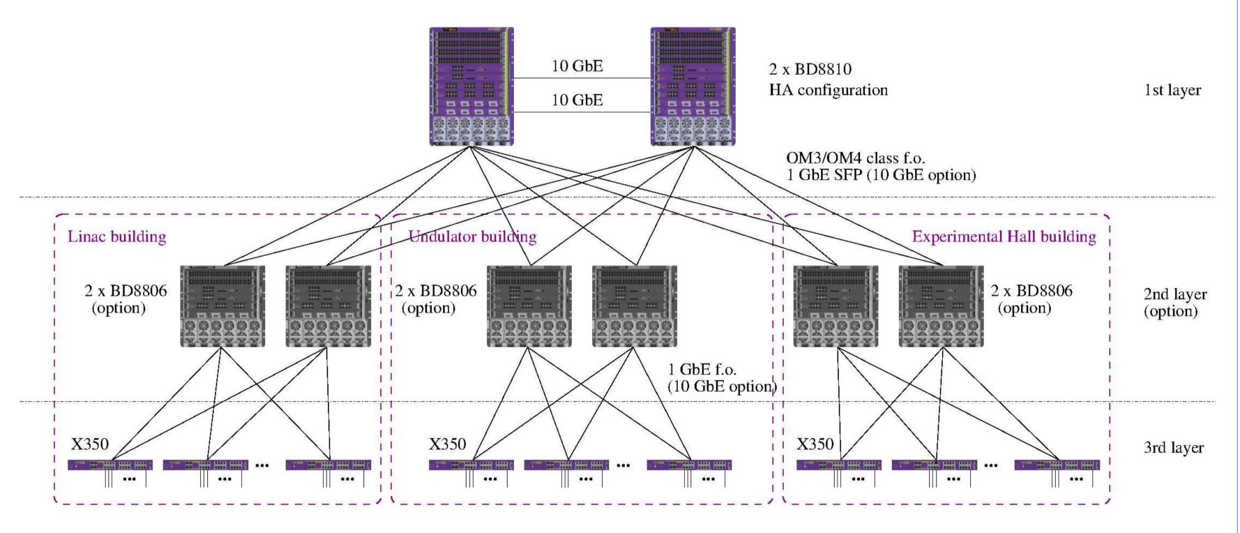
Optical Multi-mode class 3 (OM3) and class 4 (OM4) fiber optic cables, capable of 10 Gb/s (10GbE) network speed over the plant distances, connect the star center, the first and second layer peripheral switches, installed into the controls and diagnostics racks.
