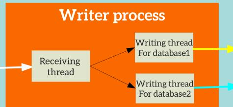
In the writer process, receiving thread publishes message to writing threads. Writing threads are separated and another thread can be added easily. It is suitable synchronous output like databases.
