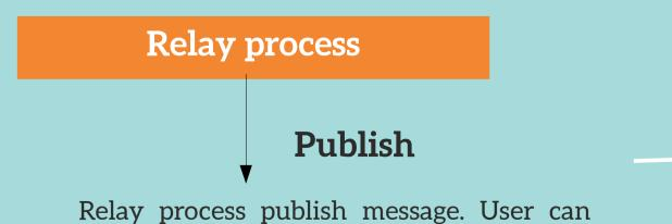
subscribe message by header keyword and signal names. For example if user want to see alarm of signal name yyzz, one can receive message by subscribing by "ALyyzz" keyword. It is suitable asynchronous application like Websocket server.
