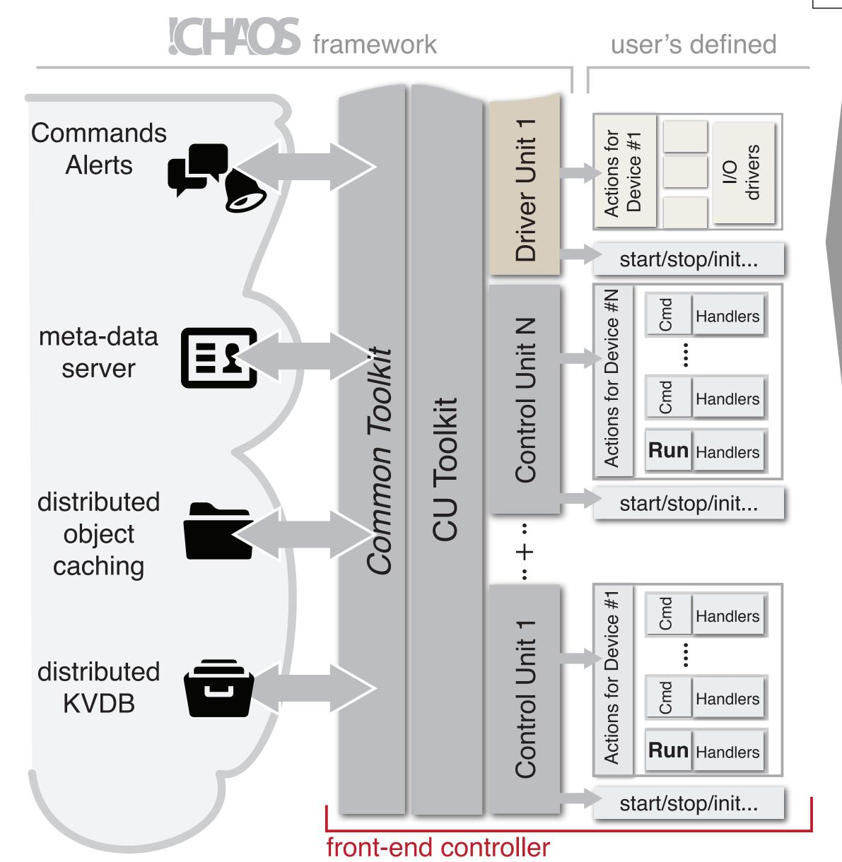
Control Unit is the "container" for a device's front-end controls. Beside the standard methods: INIT, START, STOP and DEINIT, CU specialization is provided by the device's dataset, the actions implemented for it (e.g. commands and control loop) and the drivers for I/O components (see Fig. on the left).
