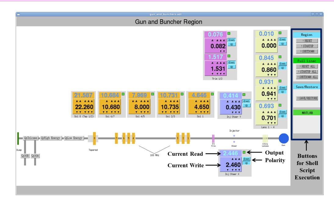
**One of the OPIs created to control the power supplies for the 44 MeV is shown** above. The current in this figure is controlled with a controller widget which has arrows. This display also runs several scripts to: turn on the output of the power supplies, reset the current value to zero, save and shutdown the power supplies, and launch a save/restore GUI with the program Back Up and **Restore Tool (BURT) for manual save/restore.**
