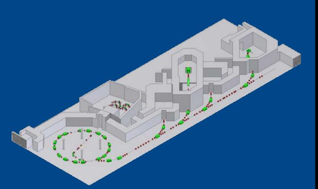
The accelerator, featuring four ion sources, IH-based Linac, synchrotron, three horizontal, one vertical beam line and one proton gantry. Energy ranges from 60 to 800 MeV/u, up to 250 MeV/u proton equivalent for ion therapy [2].
