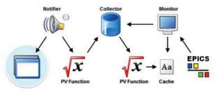
Figure 1: Architecture diagram. Shows the part of the client that runs at the rate dictated by the source of the data on the right and the part of the client that runs at the rate at a client dependent rate.
