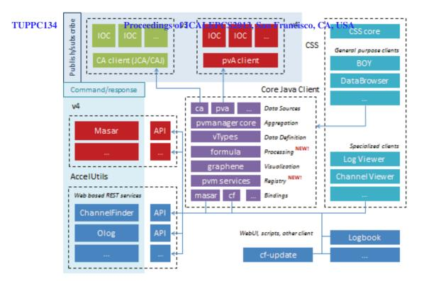
Figure 2: Overall Architecture of accelerator tools and services.
