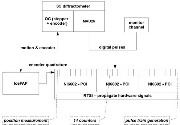
Figure 1: BL04 (MSPD) HRPD experiment. Application schema with involved instruments and controls hardware.
