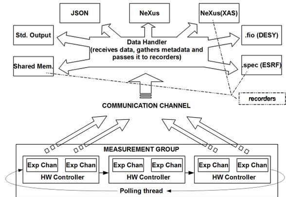
Figure 2: Data collection mechanism during the scan execution.
