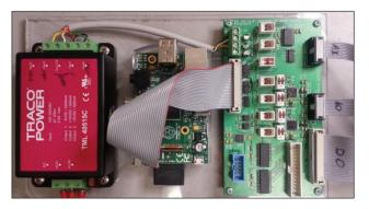
Figure 8: EPICS IOC for the control of the focalization system.
