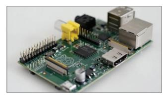
Figure 3: Raspberry Pi computer board (model B, rev. 2).
