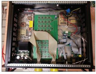
Figure 6: EPICS IOC for the control of the beam diagnostic unit.
