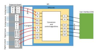
Figure 4: Interface between the EPICS IOC records and the expansion board using a C program.
