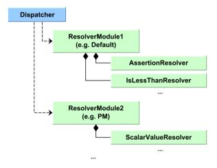
Figure 3: Relations of components involved in the resolving process (simplified).
