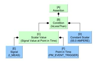
Figure 2: Expression tree created from listing 1. Characters in square brackets ([]) are labels for the nodes; blue nodes are already resolved ones (values known); green ones are unresolved (to be calculated).
