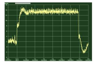
Figure 4: Cryolosses measured during the CW operation with gradient around 7MV/m.
