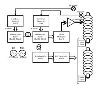
Figure 2: Former hardware setup for initial CW tests.
