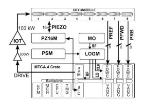
Figure 3: MTCA.4 based LLRF system configuration [2].
