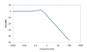
Figure 4: Transfer function for this PLL.
