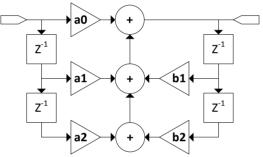
Figure 5: Infinite impulse response structure that implements the PI compensator.
