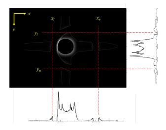
Figure 3: DM3/DM4 near field edge detection image and x- and y-projections of the edges.
