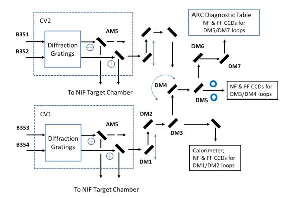
Figure 1: Simplified schematic of the beam path from the ARC compressor vessels to the ARC Diagnostic Table. NIF beams B351 and B352 are input to Compressor Vessel CV1, and beams B353 and B354 input to CV2, and a fraction of one of these beams is switched to the ARC Diagnostic Table. Labels for the DM1—3 mirrors and calorimeter package for CV2 are omitted for clarity.
