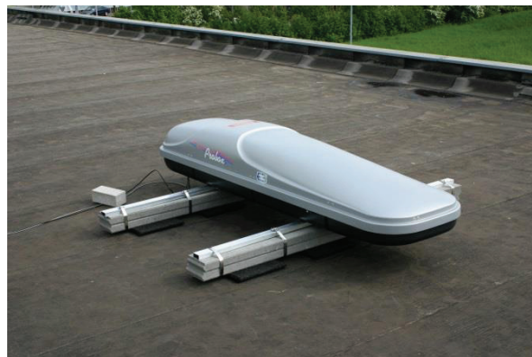
Figure 1: Typical HiSPARC detector.
