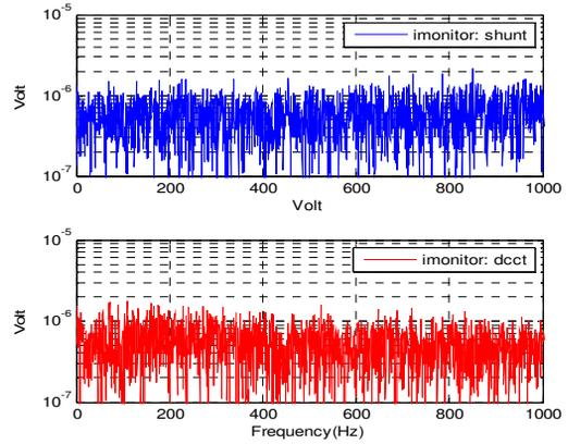
Figure 8: Noise level is around 1uA.
