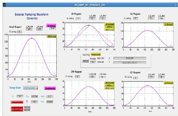
Figure 2: GUI for booster bending magnet and 4 families of quadrupoles ramping waveform generation and download.
