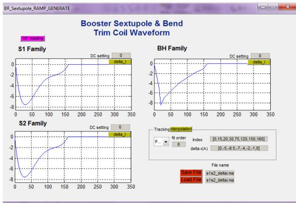
Figure 6: GUI for booster 2 families of sextupoles and bending trim coil ramping waveform generation and download.
