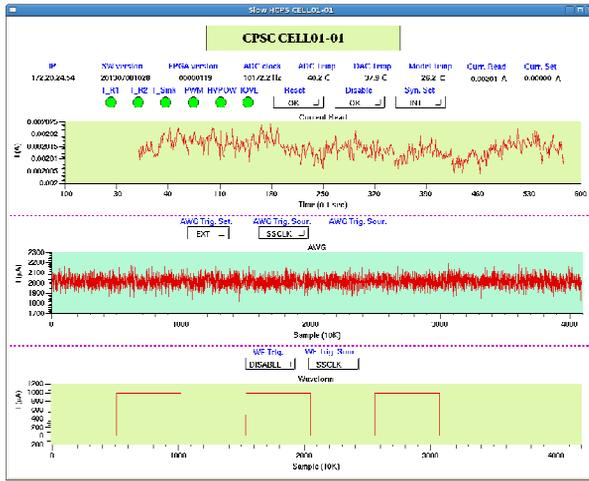
Figure 5: GUI for booster corrector controller (CPSC) control EDM page.
