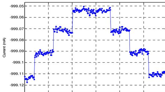
Figure 7: 20 bit performance, each step is around 20 uA.
