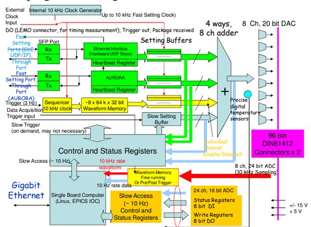
Figure 4: Functional block diagram of the corrector power supply controller (CPSC) module. It includes fast setting from orbit feedback, slow setting and waveform download from EPICS CA.
