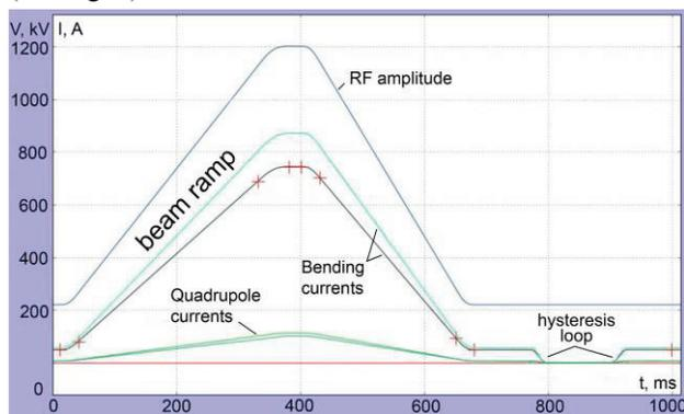
Figure 1: Ramping curves for main magnets and RF in 1 Hz cycle mode.
