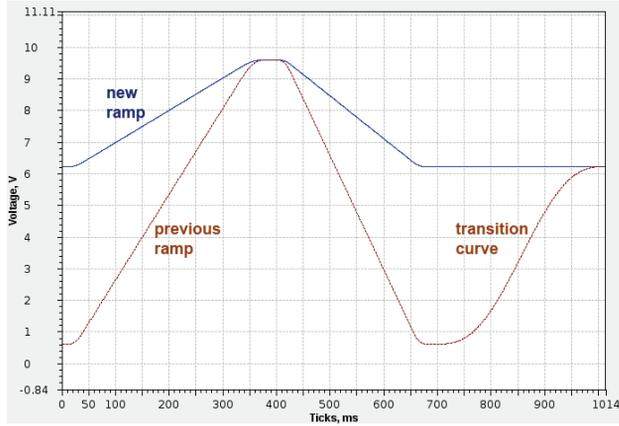
Figure 2: Ramping waveforms with the transition waveform (brown).
