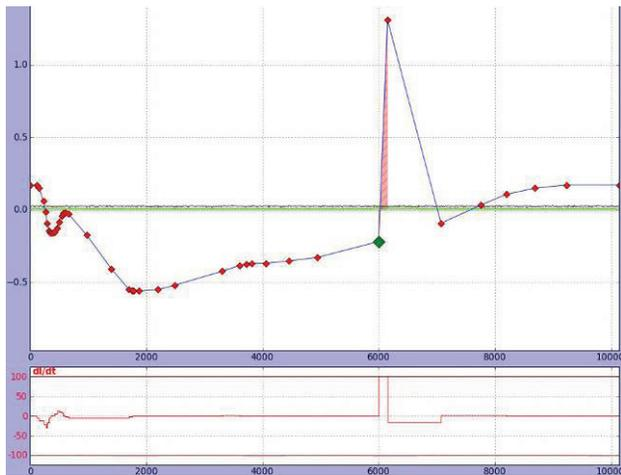
Figure 4: Ramping waveform for sextupole magnet with wrong setpoint.
