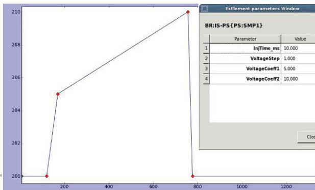
Figure 6: Reference voltage for the injection septum.
