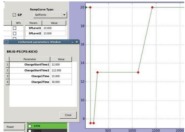
Figure 7: Reference voltage for the injection kicker.
