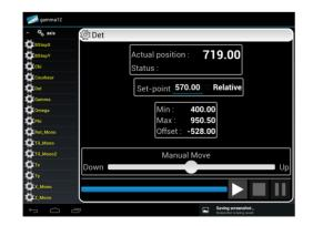
Figure 4: A tree view allows to select the desired axis and to access the new functionalities to manually control mo-
