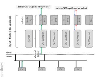
Figure 2: A schematic diagram of CAFE's multi-index container composed of two indices, the handle (or object reference) and the process variable name. CAFE methods first query the CAFEConduit object within the container, shown here to be indexed by handle, to verify the channel's current state before deciding to send a message to the CA server hosted by the IOC.
