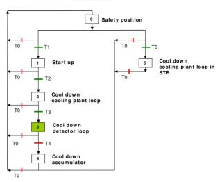
Figure 3: CO<sub>2</sub> cooling control system sequencer.
