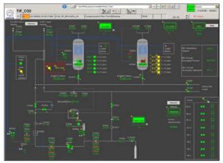
Figure 4: Main panel of the CO<sub>2</sub> cooling synoptic.
