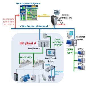
Figure 2: CO<sub>2</sub> cooling control system architecture.
