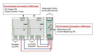
Figure 5: Redundant 24Vdc power supplies.
