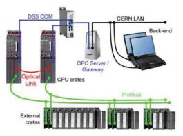
Figure 1: LHC Detector Safety System.
