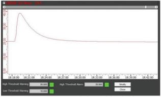
Figure 8: Temperature evolution and threshold.
