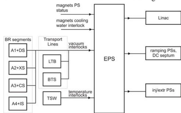
Figure 1: EPS subsystem interfaces.
