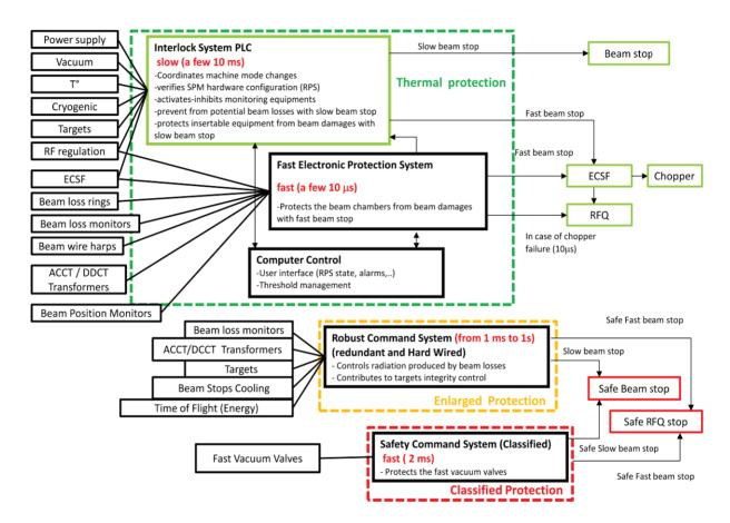
Figure 1: Functional Schem of the SPIRAL2 Machine Protection System, with its three sub-systems: Thermal Protection, Enlarged Protection, Classified protection for fast vacuum valves.
