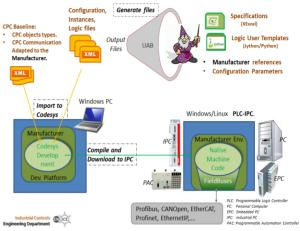
Figure 2: UNICOS-CPC CODESYS procedure.
