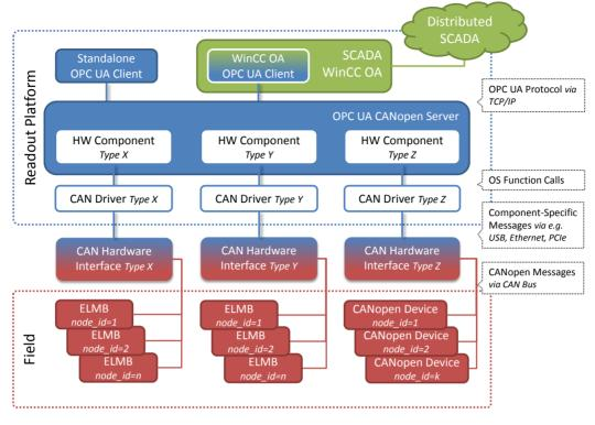
Figure 1: A schematics showing typical use case of OPC UA in the ATLAS DCS.
