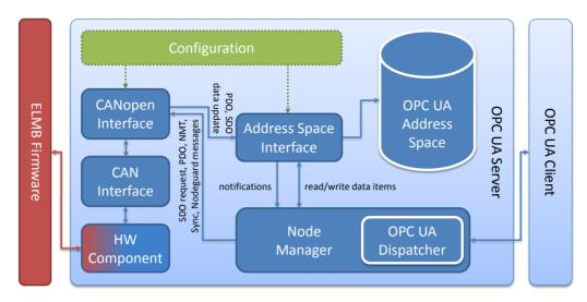
Figure 2: Software components of the server and data flow among them. CANopen specific terms like SDO, PDO, NMT are described in [2].
