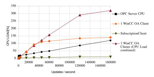
Figure 3: CPU load of OPC UA software components vs few update rate values.
