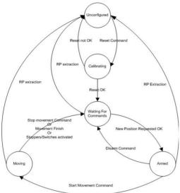
Figure 6: The enhanced state machine, as prototyped and validated on the testbench.
