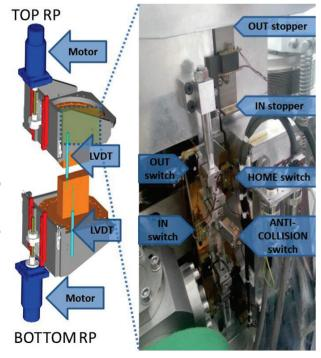
Figure 2: The Roman Pot Front End, sensors and actuators.
