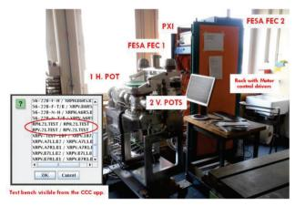
Figure 4: The testbench - a clone of the production system.
