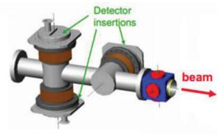
Figure 1: 2 Vertical and 1 Horizontal Roman Pot on the LHC beam pipe.
