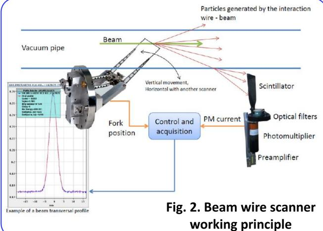
**Fig. 2. Beam wire scanner working principle**
