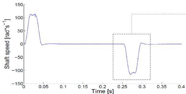
**Fig. 4. Shaft speed with 6 superimposed scan cycles**
