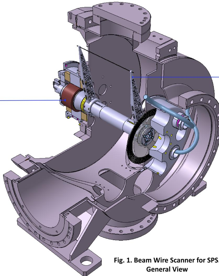
**Fig. 1. Beam Wire Scanner for SPS. General View**
