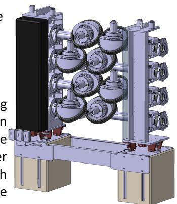
**Fig. 7. Integration of the beam wire scanner in PSB**
