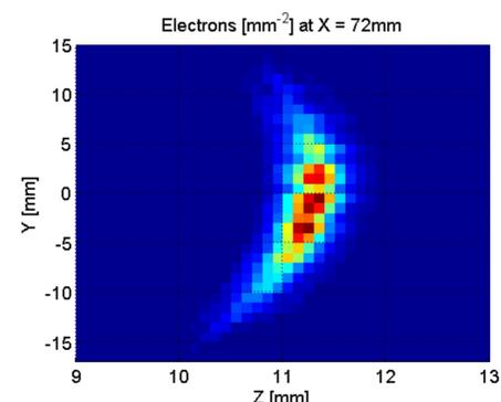
Expected electrons distribution at the detector plane, accounting for all laser positions during a scan.
