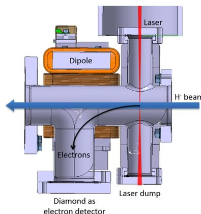
The laser beam diameter is relatively small with respect to the H<sup>-</sup> beam size, hence the vertical position of the liberated electrons is well defined and counting the stripped electrons as function of the laser position during a scan allows to reconstruct the beam profile.
