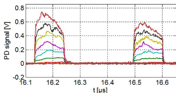
Laser pulses with different energies before (left) and after fiber (right)
