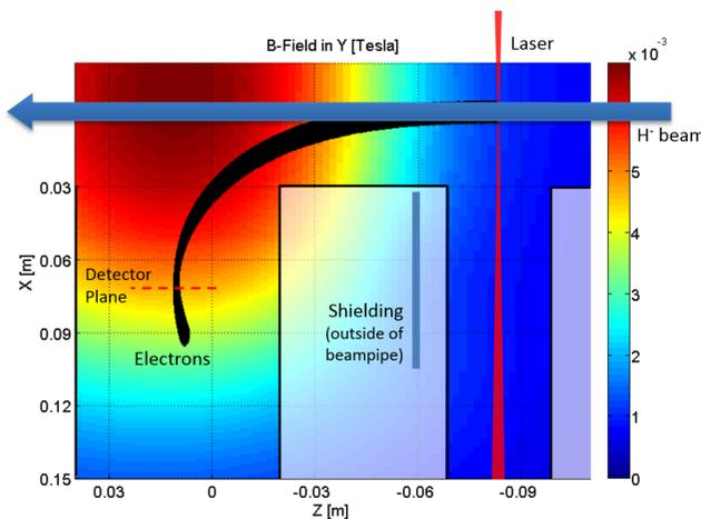
Magnetic field map and electron trajectories (black) from the laser interaction point to the diamond detector at X = 72 mm.
