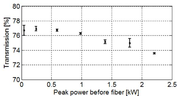
Laser transmission through the 75m LMA optical fiber
