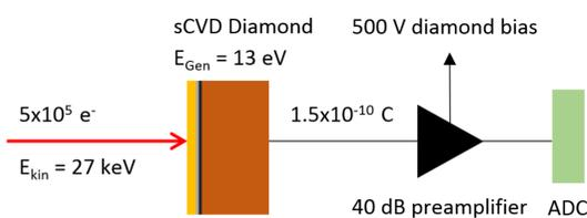
Signal creation and readout of diamond detector
