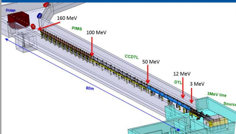
The LINAC4 commissioning is taking place in stages at different beam energies. During the 3/12 MeV commissioning, a non-invasive laser system was successfully operated to measure the vertical emittance of the H<sup>-</sup> beam, by collecting the neutralized H<sup>0</sup> atoms.
