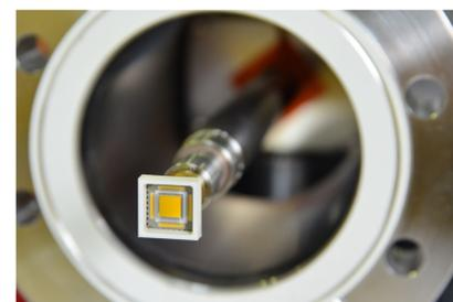
sCVD diamond detector mounted on the vertical actuator
