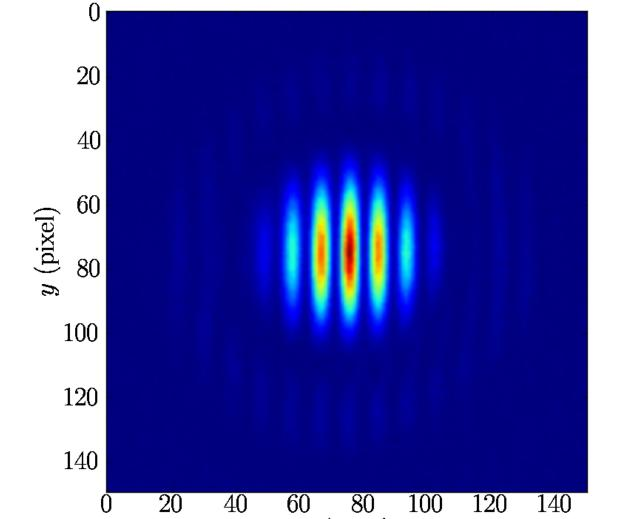
Because this aperture, the light reaching Xanadu is creating a blurring of the image due to the curvature of the trajectory. The bending radius of the magnet producing the radiation is 7.05 m, that leads to blurring of  $\pm 13 \mu$ m. This incoherent effect can be observed when measuring the horizontal beam size using the pinholes distance scan.
